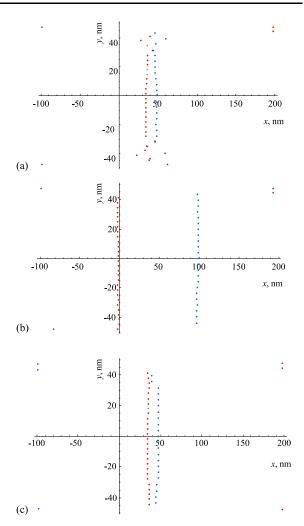
**Fig. 4.** Characteristic equilibrium profiles of migrating low-angle GBs in the third migration mode.  $\sigma = 30^{\circ}$ ,  $\sigma = 1.9$  GPa, M(x, y) = (-L, -L/2), l = 15L. (a) In the first loading cycle, all dislocations reach equilibrium positions or high-angle GBs. (b) During unloading after the first cycle of loading, dislocations not captured by high-angle GBs tend to return to their initial positions. (c) Under a new loading cycle, new dislocations migrate to high-angle GBs.
