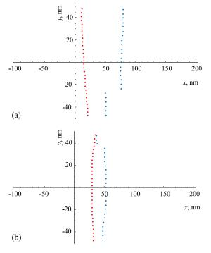
**Fig. 3.** Characteristic equilibrium profiles of migrating low-angle grain boundaries in the second migration mode. (a)  $\alpha = 45^{\circ}$ ,  $\sigma = 1.6$  GPa, M(x, y) = (L, L/2), l = 15L; (b)  $\alpha = 30^{\circ}$ ,  $\sigma = 1.1$  GPa, M(x, y) = (-L, -L/2), l = 30L.
