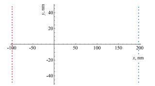
**Fig. 8.** Characteristic equilibrium profiles of migrating low-angle grain boundaries in the seventh migration mode.  $\alpha = 45^{\circ}$ ,  $\sigma = 1.8$  GPa, M(x, y) = (-L, -L/2), l = 30L.
