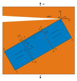
**Fig. 1.** Collective migration of low-angle grain boundaries under the action of an external load in a nanocrystalline metal.
